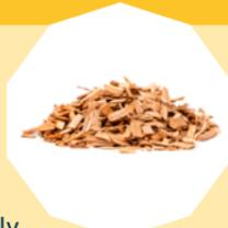
Wood is needed to produce silicon metal and silicon-based alloys. Wood chips are used directly in furnaces. 100% of the wood chips used in our production processes are purchased externally. In South Africa, where the main source of carbon reductant is charcoal, wood logs are purchased and transformed into charcoal.
