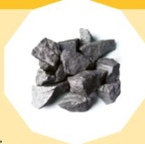
Manganese ore is used to produce manganese-based alloys in our plants in France, Norway and Spain.
